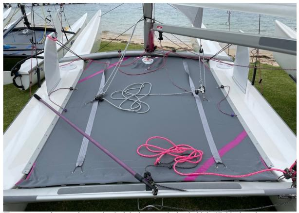
There are no wires or other mechanical devices attached to hold the jib block to the trampoline. It is simply attached to the rope loop and the eyelets are through sufficient reinforcing on the trampoline to cater for the jib sheet load. The cost to update an existing trampoline is \$200. No need to buy a new trampoline.
