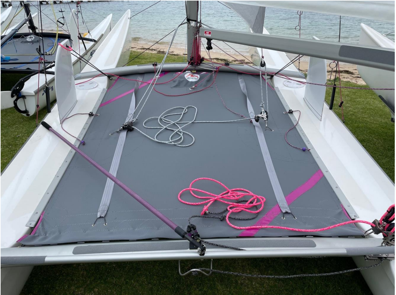
Photo 4.2: There are no wires or other mechanical devices attached to hold the jib block to the trampoline. It is simply attached to the rope loop and the eyelets are through sufficient reinforcing on the trampoline to cater for the jib sheet load. The cost to update an existing trampoline is $200. No need to buy a new trampoline.
