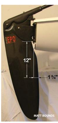
Rudder toe in should be 1/8" with the rudders in the locked down position again measured from the 12" down point. "Toe-in" means that the leading edges are closer together than the trailing edges.
