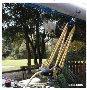
Instead of rivets to attach the boom bail, I use a through bolt that allows the bail to pivot with the changing angle of the mainsheet.
