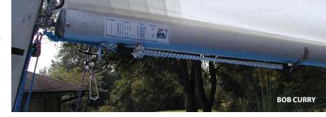
CURRY: There are a lot of different thoughts on this area. I will address what has worked for me. The basic, optimal sail shape has its maximum draft position at 45% aft and the maximum draft is 16% of the chord length.
