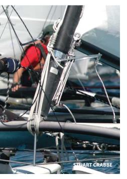
HOTLINE: If you capsize with a loose rig, there is a good possibility the mast could come out of the step, making righting difficult and a tow to shore necessary. To prevent this, wrap the halyard in a figure-8 pattern around the dolphin striker and the cleat and lash it together as shown in the photo.
