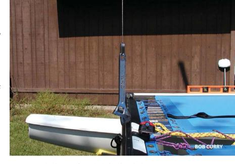
Measure the distance from the halyard to the bottom of the mast cutout for the mainsail. A good ball park number will range between 45"–57" depending on your body weight. Lighter skippers will favor the larger number (more mast rake) and heavier skippers will favor the smaller numbers (less mast rake). Since I weigh 160 lbs, I opt for a 55" mast rake.
