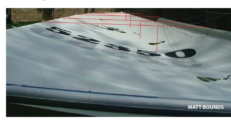
**HOTLINE**: If you have access to photo editing software, like PhotoShop, you can measure the position and amount of maximum draft by taking photos of the sail, then drawing / measuring the draft lines on the computer.
