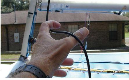
As the breeze freshens, I tighten the rig to keep the leeward hull from depressing too much. This is very important to remember in choppy water. When trapezing, adjust the shroud tension to 45 degrees using the same described previously. This will keep the rig powered up and not dump you in the water in lulls.
