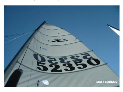
*CURRY*: I tension the battens starting from the bottom and working to the top. This is done with the sail lying on the trampoline:
