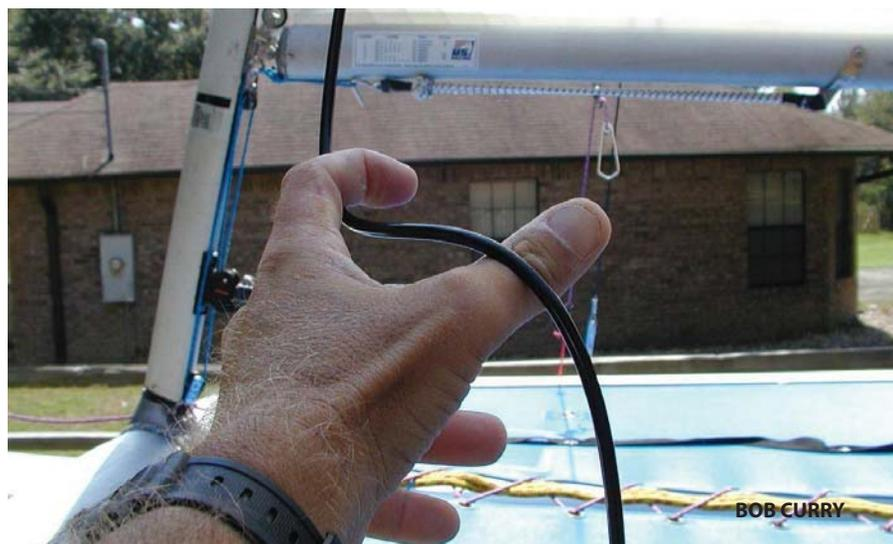
As the breeze freshens, I tighten the rig to keep the leeward hull from depressing too much. This is very important to remember in choppy water. When trapezing, adjust the shroud tension to 45 degrees using the same described previously. This will keep the rig powered up and not dump you in the water in lulls.
