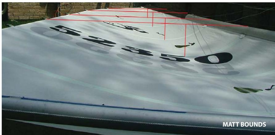
**HOTLINE:** If you have access to photo editing software, like PhotoShop, you can measure the position and amount of maximum draft by taking photos of the sail, then drawing / measuring the draft lines on the computer.
